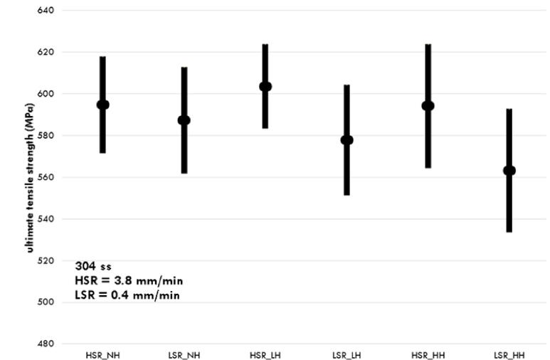
Figure 2 shows ultimate tensile strength data for 304 stainless steel specimens that were tested at two strain rates. The abscissa axis indicates the strain rate and hydrogen exposure conditions. The dot in the middle of each vertical bar on the graph is the average tensile strength for the samples that received the given strain rate and hydrogen exposure treatment. The length of the bar indicates plus or minus one standard deviation from the mean.
