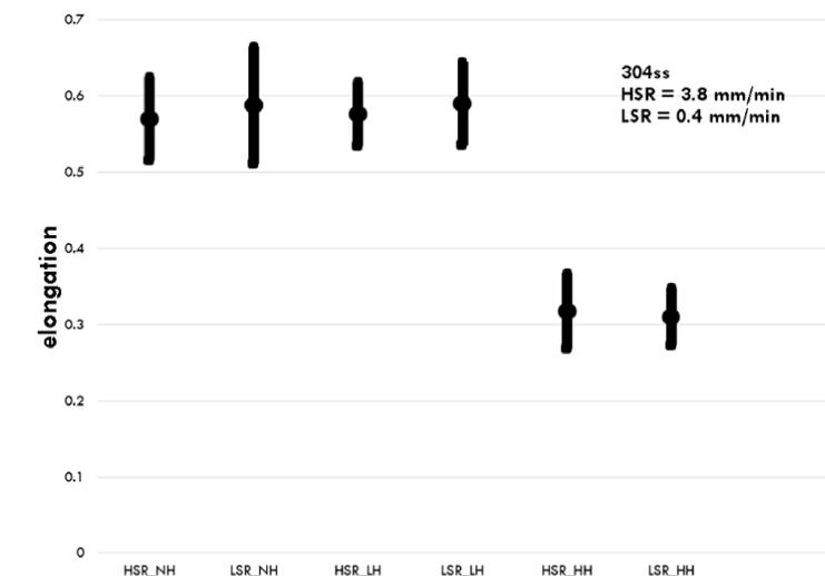
Fig. 3 Elongation for 304 stainless tensile specimens for three different hydrogen exposure levels, tested to failure at two different strain rates. The data shows that the elongation of the supersaturated specimens (aka 'high hydrogen') is lower than that of the other exposure conditions (no hydrogen and low hydrogen).
