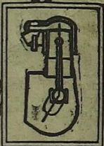
Rambler Offset Crank Shaft. Position of crank shaft at explo- sion center.
