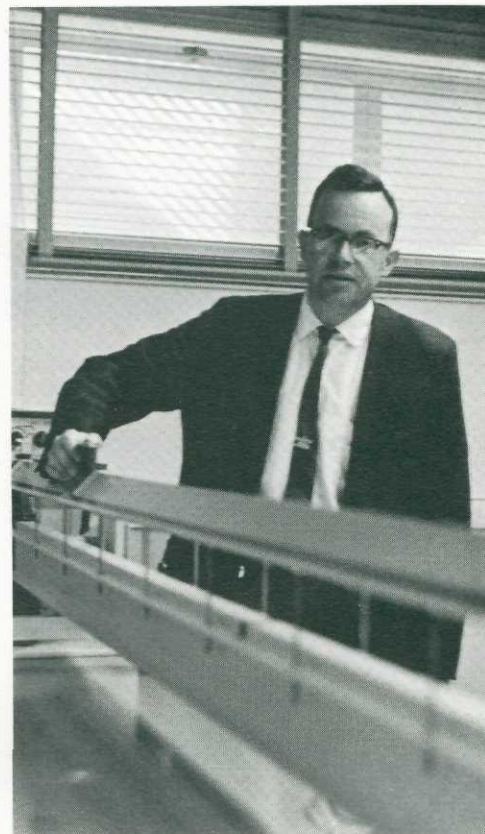
Above: Dr. Johnston demonstrates the friction-foiling airtrack, utilizing a non-drag aircushion.
