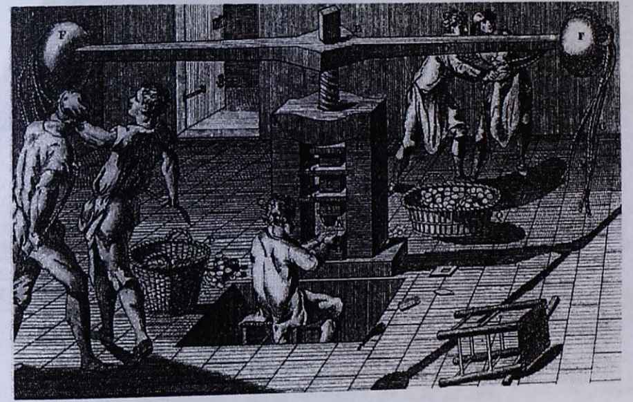
Illustration 57. Engraving, plate XV from Diderot's and d'Alembert's Encyclopédie , depicting an eighteenth-century screw press. From Cohen, 30.
